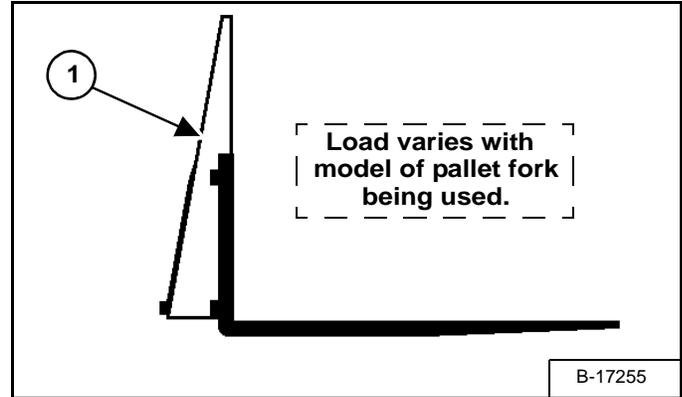
If a pallet fork attachment is used, the load center moves forward and reduces the load capacity.
