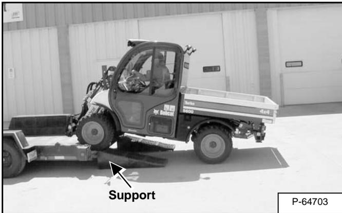
A machine with an attachment must be loaded or unloaded forward. A machine without an attachment can be loaded or unloaded either forward or backward [Figure OI-80].
