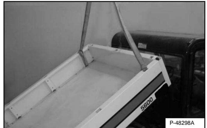
Install lift straps (or chains) through the stake holes at the front of the cargo box [Figure PM-10].
