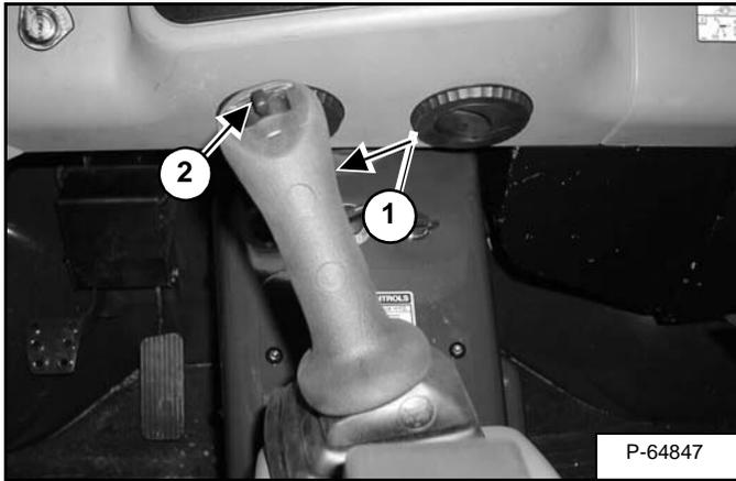
The trigger switch (Item 1) [Figure OI-26] on the front of the joystick can be used for continuous flow. Move the thumb switch (Item 2) [Figure OI-26] to the desired direction, then press and release the trigger switch. Release the thumb switch.
