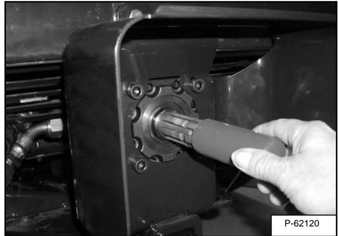
Put the plastic sleeve on the PTO shaft [Figure OI-41] to prevent dirt and debris from collecting on the PTO shaft splines.
