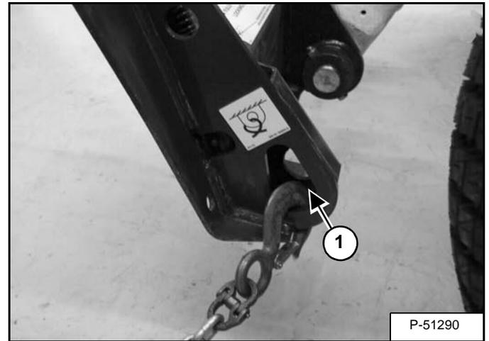
Fasten chains at the front using the tie down holes in the Bob-Tach (Item 1) [Figure OI-82].
