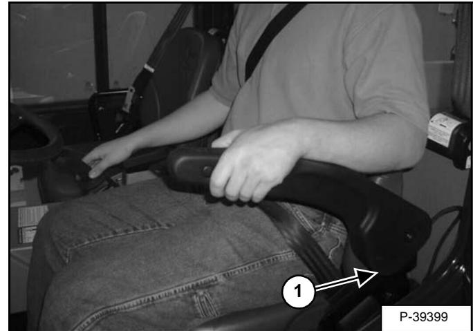
Use compressed air to clean any debris or dirt from the pivot parts (Item 1) [Figure PM-2]. Do not lubricate. Inspect all mounting hardware and tighten as necessary.
