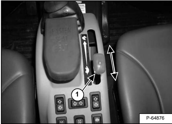
The engine speed control (Item 1) [Figure OI-9] is on the center console at the right side of the operator's seat. Move the engine speed control forward to increase the engine RPM and backward to decrease.
