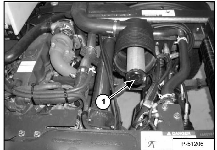
Remove the outer filter element (Item 1) [Figure PM-18] and, if required, remove the inner element (Item 1) [Figure PM-19].
