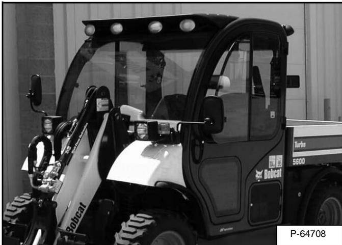
The machine has an operator cab (ROPS and FOPS) [Figure PM-12] as standard equipment to protect the operator from rollover and falling objects. The seat belt must be worn for rollover protection. Check with your dealer if the operator cab has been damaged or modified.
