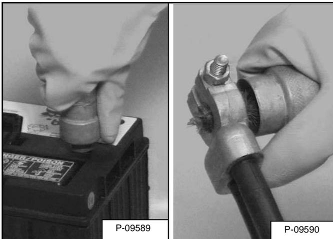
Always clean the battery terminals and cable ends when installing a new or used battery [Figure PM-36].
