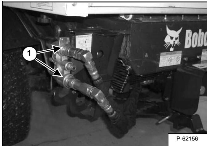
To connect the PTO motor, remove the hoses from the storage hooks. Connect the quick couplers (Item 1) [Figure OI-28] to the rear auxiliary hydraulics by pressing the couplers together until they securely latch. (See REAR AUXILIARY HYDRAULICS (If Equipped) on Page OI-17.)
