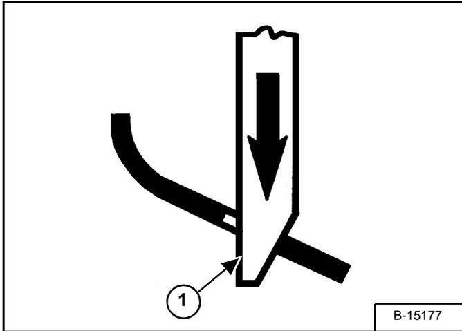
The wedges (Item 1) [Figure OI-67] must extend through the holes in the mounting frame of the bucket (or attachment), securely fastening the bucket or attachment to the Bob-Tach.
