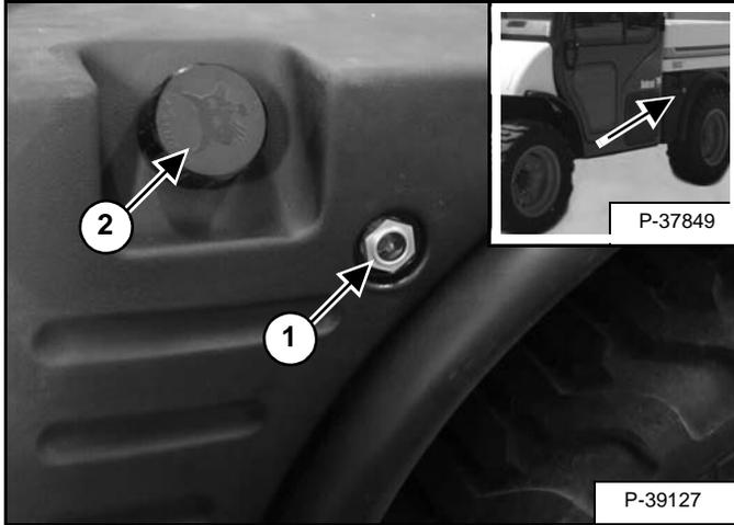
Check the fluid level in the sight gauge (Item 1) [Figure PM-39]. The fluid level is correct when at the center of the sight gauge.
