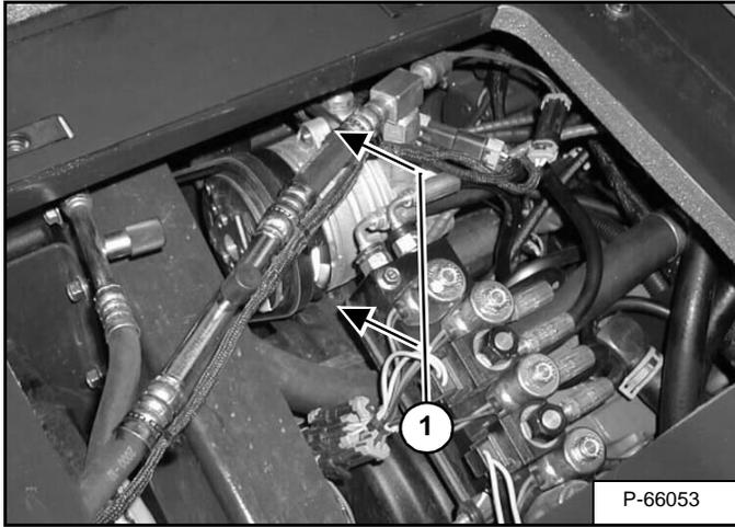
Loosen adjustment and mounting bolts (Item 1) [Figure PM-51].
