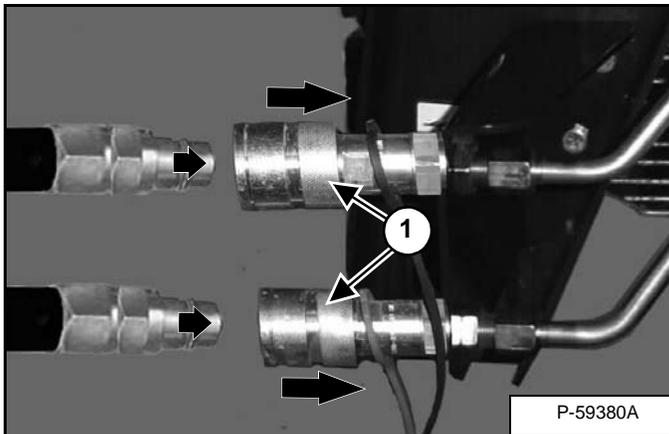
*To Connect:* Pull back on the collar of the female couplers (Item 1) [Figure OI-46]. Push couplers together, release the collar when the couplers are fully engaged and locked.
