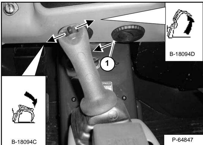
The thumb switch on the joystick now controls the front auxiliary hydraulic functions.
