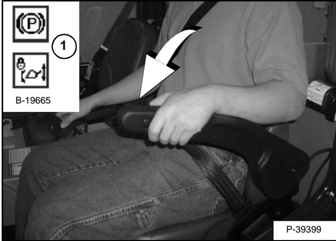
The TICS requires the operator to be seated in the operating position with the arm rest [Figure OI-7] fully lowered before the lift, tilt and traction functions can be operated. The seat belt must be fastened anytime you operate or are a passenger riding in the machine.
