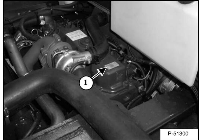
The engine serial number is located at the right end of the valve cover (Item 1) [Figure 2].
