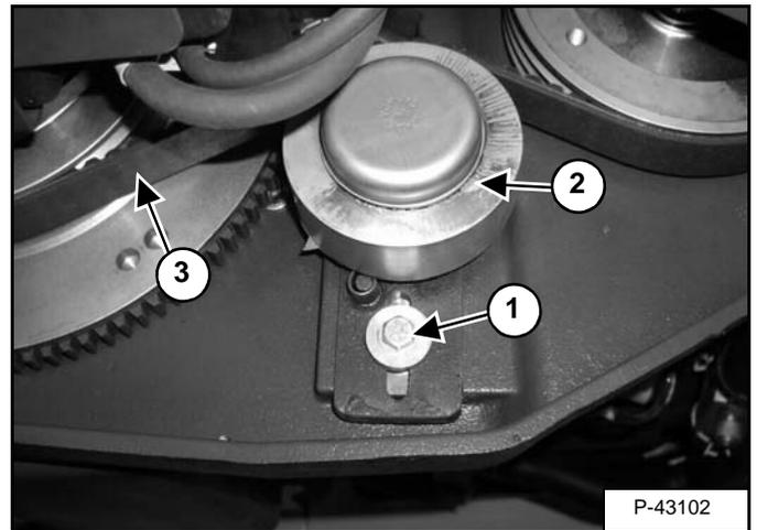
Loosen and remove the bolt (Item 1) [Figure PM-56] from the belt tensioner.
