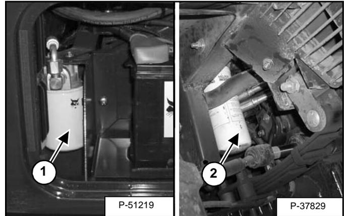
Remove the case drain filter (Item 1) [Figure PM-40].
