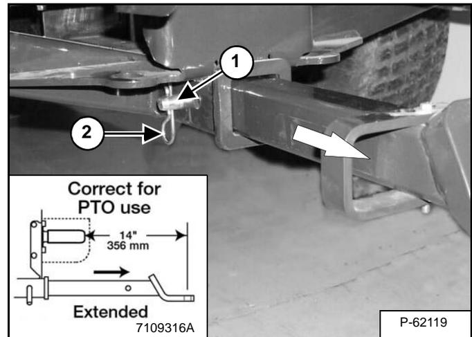
Extend the receiver hitch to the position shown (Inset) [Figure OI-30]. Install the receiver hitch pin in the hole (Item 1) and secure it with the retaining pin (Item 2) [Figure OI-30].
