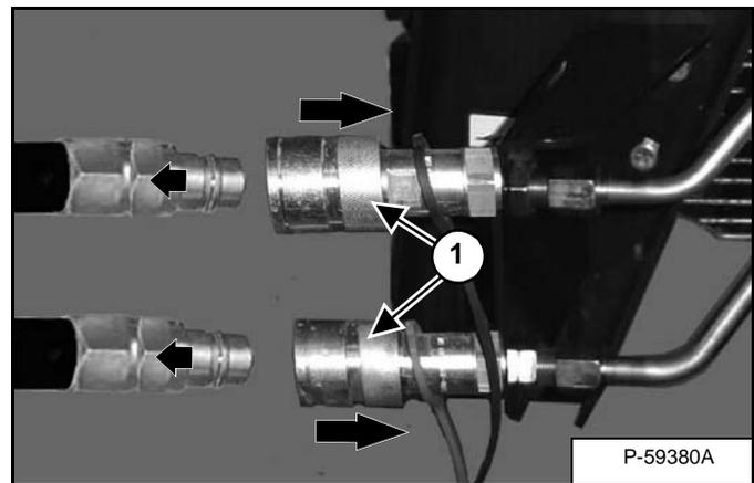
*To Disconnect:* Pull back on the collar (Item 1) [Figure OI-48] and pull the male coupler out to disconnect.
