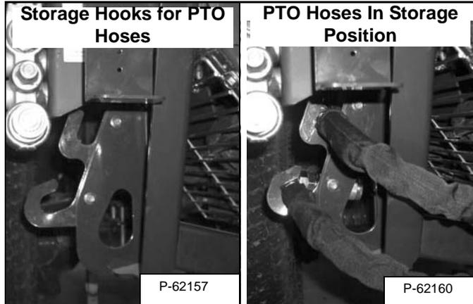
When the PTO motor quick couplers are disconnected, they can be stored in the hooks provided at the rear of the machine [Figure OI-27].
