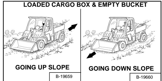
With empty bucket and a loaded cargo box, go down or up the slope with the heavy end toward the top of the slope [Figure OI-71].
