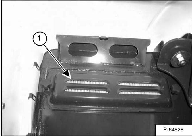
The fresh air filter is located under the right front fender [Figure PM-14].
