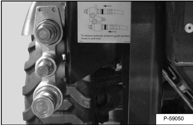
The quick couplers are located under the left side of the cargo box near the rear of the machine [Figure OI-23].
