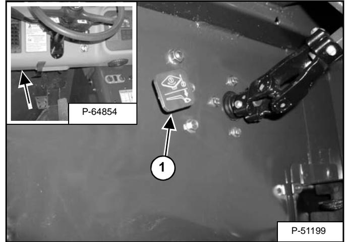
The lift arm by-pass is used to lower the lift arm in the event that you cannot lower the lift arm using the joystick.
