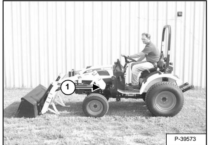
Remove the drain plug at the bottom of the differential (Item 1) [Figure PM-49].
