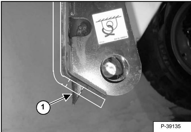
The wedges must extend through the holes in the attachment mounting frame (Item 1) [Figure PM-68].
