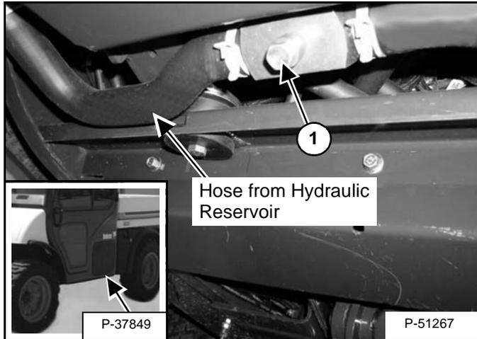
Remove the plug (Item 1) [Figure PM-41] from the fitting under the front end of the cargo box.
