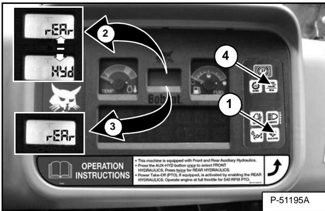
Press the auxiliary hydraulics button (Item 1) twice to activate the rear auxiliary hydraulics. The words **rEAR** then **Hyd** (Item 2) will flash several times on the display.
