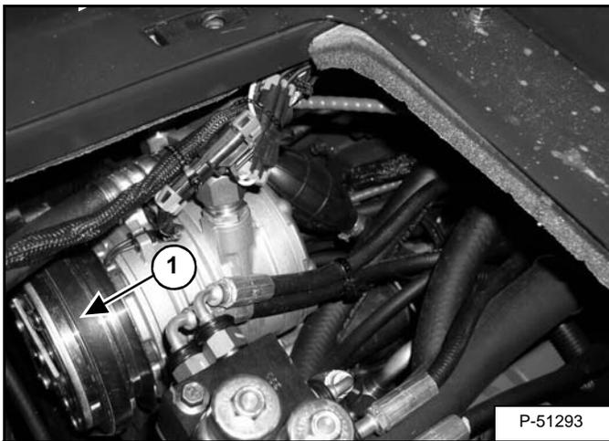
Remove the air conditioner compressor drive belt (Item 1) [Figure PM-55] (If equipped).
