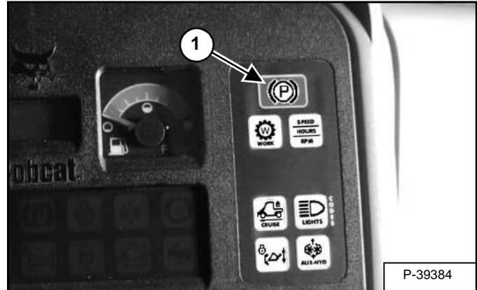
Press the button (Item 1) [Figure OI-10] to engage the parking brake. If the button is pressed, you must press it again to disengage.
