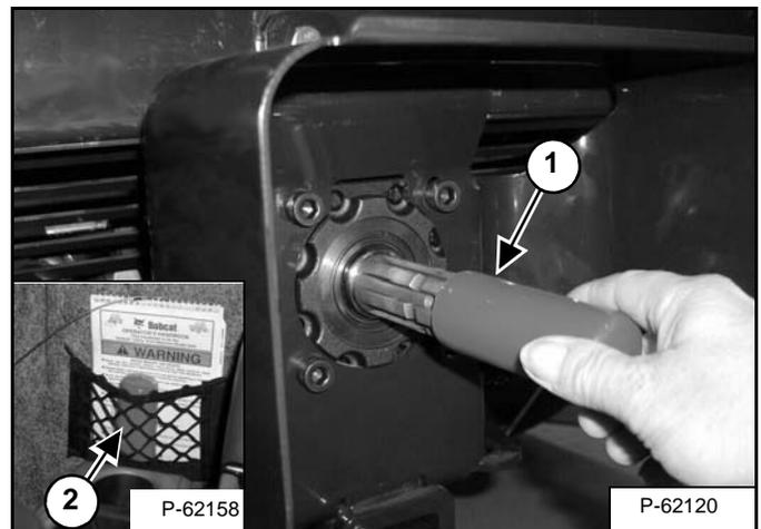
Remove the plastic PTO shaft sleeve (Item 1) [Figure OI-33]. Keep the sleeve for use later when no PTO driveline is attached. It keeps dirt and debris off the shaft splines. Store the sleeve in the Handbook pouch (Item 2) [Figure OI-33] in the cab of the machine.
