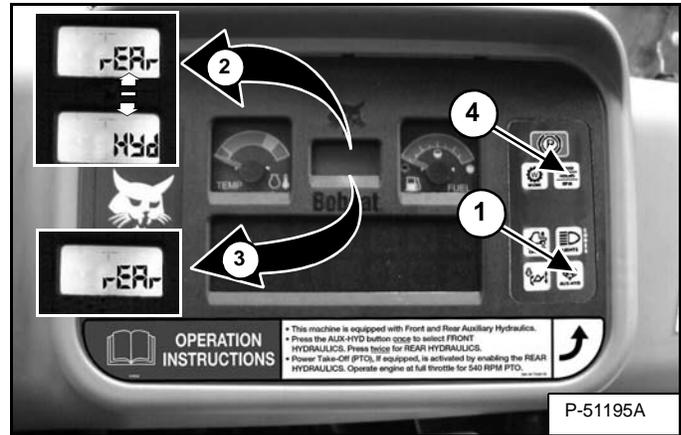
Press the Auxiliary Hydraulics button (Item 1) twice to activate the Rear Auxiliary Hydraulics/PTO. The words **rEAR then Hyd** (Item 2) will flash several times on the display. After a few seconds, the word **rEAR** (Item 3) [Figure OI-36] will remain on the display.
