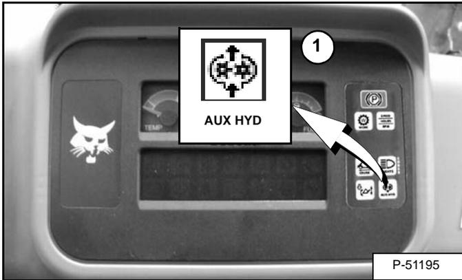
Press the auxiliary hydraulics button (Item 1) [Figure OI-19] to activate the front auxiliary hydraulics.
