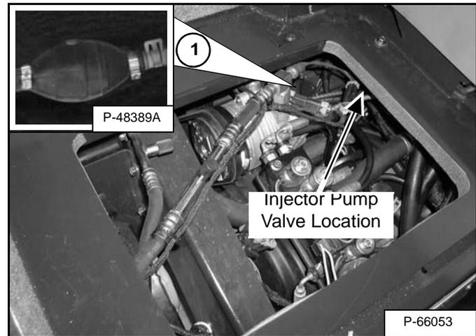
Open the valve (Item 1) [Figure PM-23] on the injector pump and squeeze the hand pump (Item 1) [Figure PM-24] several times until fuel comes from the valve with no air bubbles.
