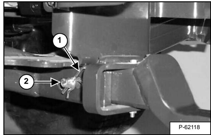
Remove the retaining pin (Item 1) [Figure OI-29] and then remove the receiver hitch pin (Item 2) [Figure OI-29].
