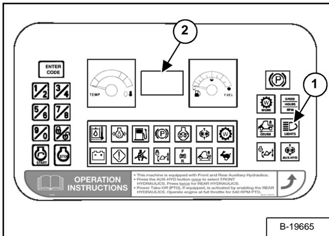
Turn the key on (Key Switch) or press ENTER CODE (Keyless). Press and hold the LIGHTS Button (Item 1) [Figure SA-1] for two seconds to view SERVICE CODES in the HOURMETER/CODE DISPLAY (Item 2) [Figure SA-1]. If more than one SERVICE CODE is present, the codes will scroll on the HOURMETER/CODE DISPLAY.
