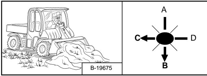
Raise the lift arm (Item B) and tilt the bucket backward (Item C) [Figure OI-73].
