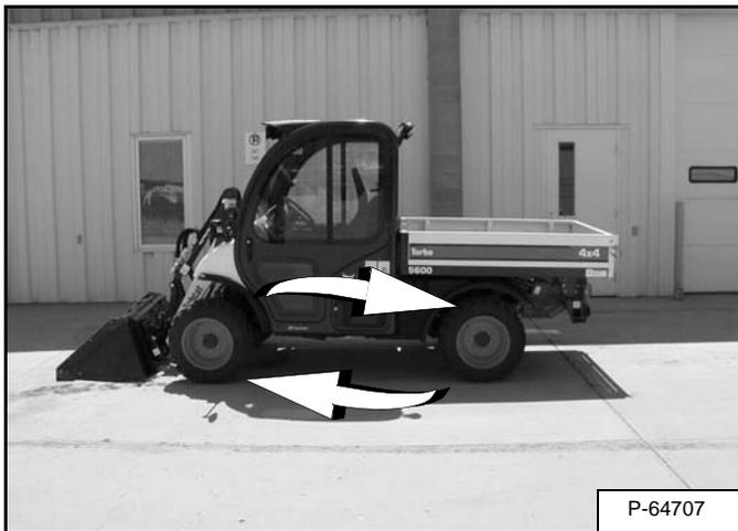
Rear tires usually wear faster than front tires. To keep tire wear even, move the front tires to the rear and rear tires to the front [Figure PM-46].
