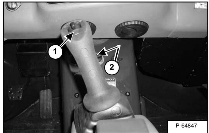
The switches on the joystick now control the rear auxiliary hydraulic functions (and PTO if equipped and connected).
