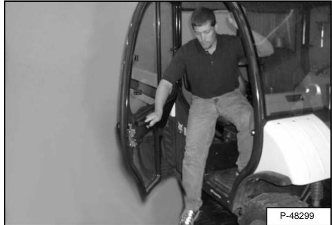
The cab door on the opposite side of the machine is used as an emergency exit [Figure OI-60].
