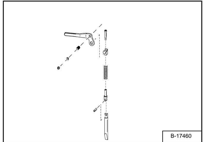
Inspect the mounting frame on the attachment and Bob-Tach, linkages and wedges for excessive wear or damage [Figure PM-69]. Replace any parts that are damaged, bent or missing. Look for cracked welds. Keep all fasteners tight. Contact your Bobcat dealer for repair or replacement parts.
