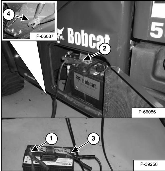
Connect the end of the first cable (Item 1) [Figure PM-37] to the positive (+) terminal of the booster battery. Connect the other end of the same cable (Item 2) [Figure PM-37] to the positive terminal of the machine battery.
