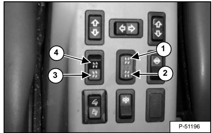
The steering mode can be selected either for Front Wheel Steer or All Wheel Steer operation.
