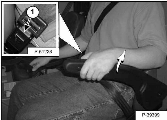
Press the red release button (Item 1) [Figure OI-59] to disconnect the seat belt.
