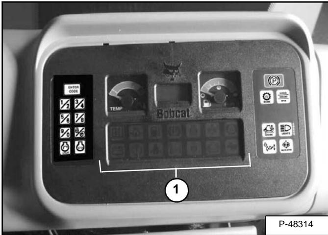
After the engine is running, frequently monitor the display controller panel [Figure OI-57] for error conditions.
