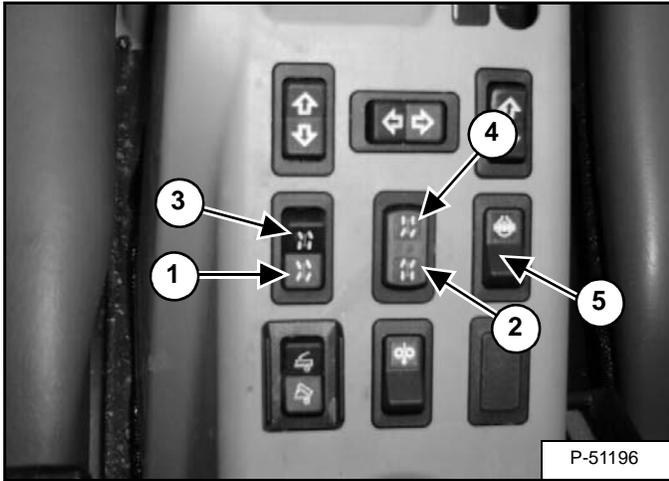
Put the Steering Mode Switch in All-Wheel-Steer (Item 1) [Figure OI-15].
