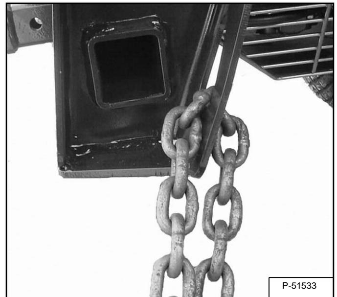
Fasten the rear of machine using the receiver hitch frame [Figure OI-83].
