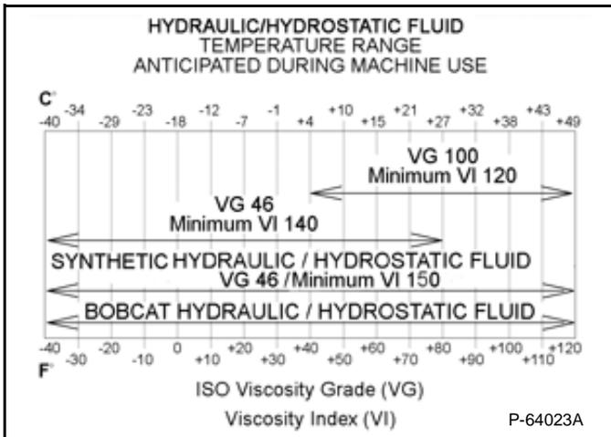
If needed, remove the fill cap (Item 2) [Figure PM-39] and add fluid. (See chart above.)
