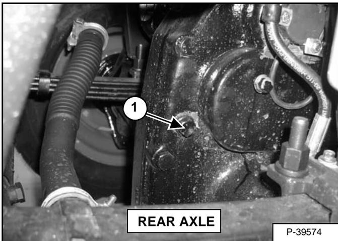
Remove the check plug (Item 1) [Figure PM-47] & [Figure PM-48] from the front or rear housing.
