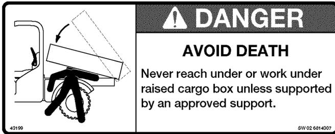
Raise the cargo box and install the approved cargo box support device. (See CARGO BOX SUPPORT DEVICE on Page PM-13.)
