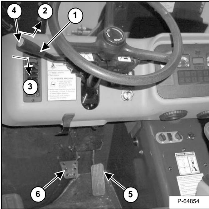
The Travel Direction Control Lever (Item 1) [Figure OI-13] has three positions; Forward - PARK - Reverse (FPR).
