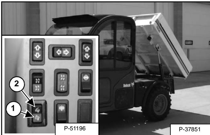
Press the back of the switch (Item 1) [Figure OI-79] to raise the cargo box. Press the front of the switch (Item 2) [Figure OI-79] to lower.
