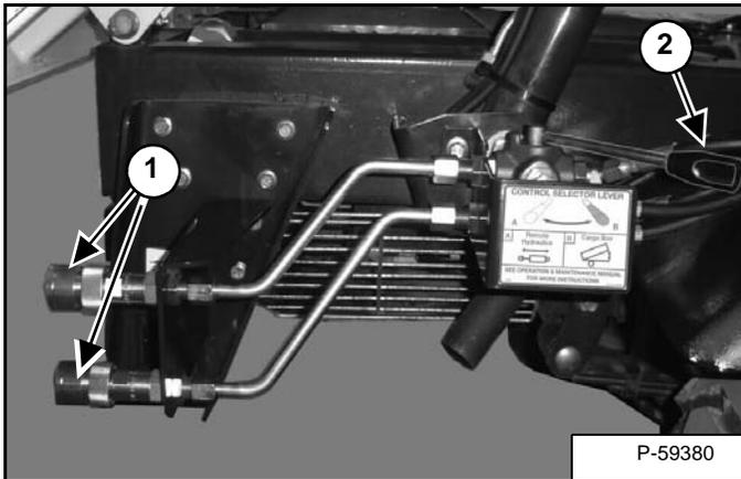
The quick couplers (Item 1) and the selector valve (Item 2) are mounted under the right side of the cargo box at the rear of the machine [Figure OI-42].
