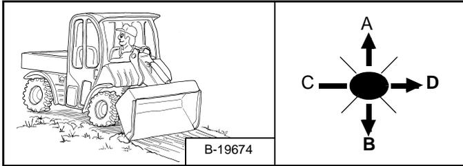
Raise the lift arm (Item B) and tilt the bucket forward (Item D) [Figure OI-75].
