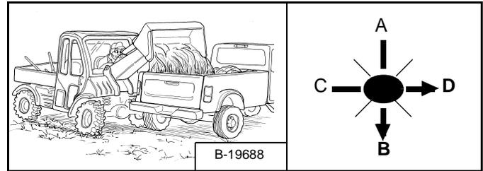
While raising the lift arm (Item B), tilt the bucket forward (Item D) [Figure OI-74] to keep it level and help prevent material from falling off the back of the bucket.
