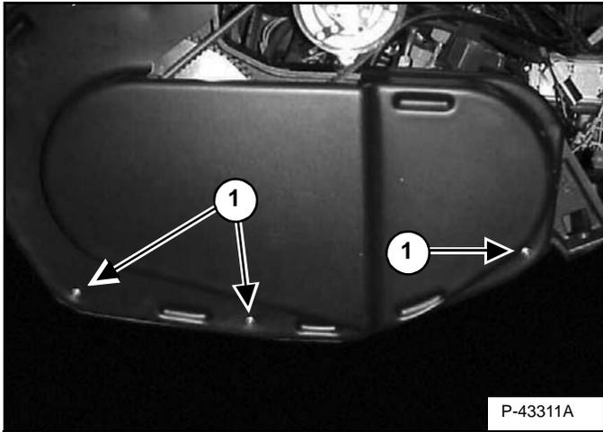
Remove the belt shield [Figure PM-52].
