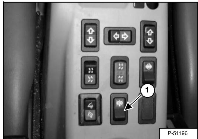
After auxiliary hydraulics is activated (Item 1) [Figure OI-21], press the high flow switch (Item 1) [Figure OI-22] on the center console. (The High Flow Icon on the switch will be ON.)
