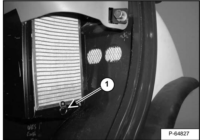
The recirculating filter is located on the right end of the heater / air conditioning housing.
