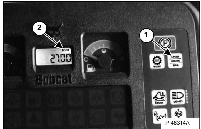
To Set 2700 RPM Engine Speed: Press SPEED/HOURS/RPM button (Item 1) [Figure OI-39] until RPM appears in display (Item 2) [Figure OI-39].
