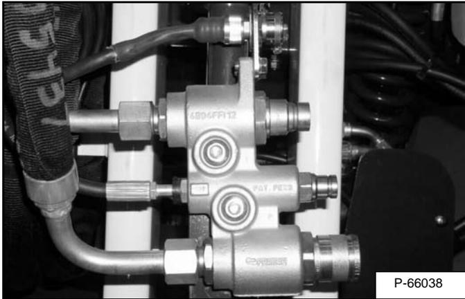
Front auxiliary hydraulics [Figure OI-18] are standard.
