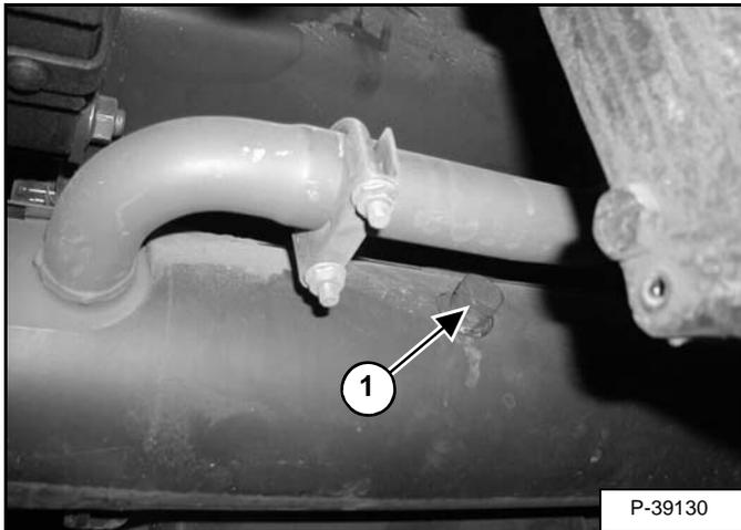
Remove the plug (Item 1) [Figure PM-43] from the cleanout hole in the muffler.
