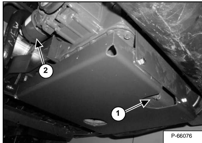
The engine oil drain and filter are located under the machine at the front end of the cargo box.
