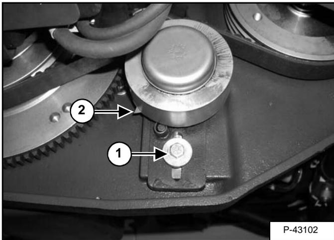
Loosen the bolt (Item 1) [Figure PM-53] on the spring loaded drive idler.
