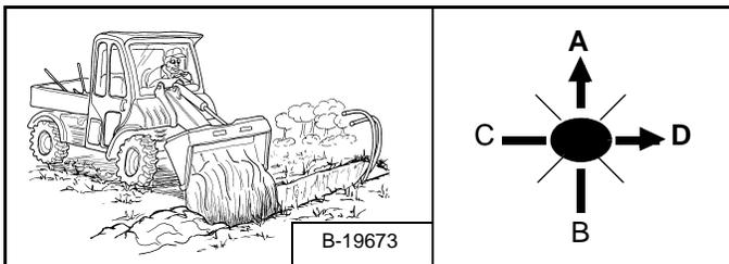
Lower the lift arm (Item A) [Figure OI-76] and put the cutting edge of the bucket on the ground (Item D) [Figure OI-76]. Drive forward to the edge of the hole to push the material into the hole.
