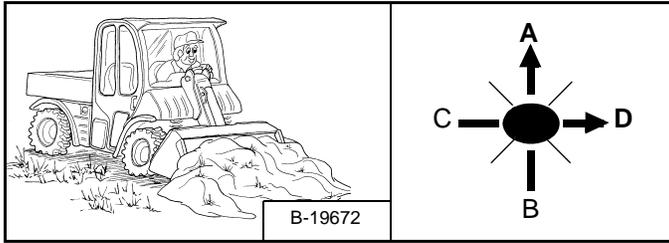
Lower the lift arm all the way (Item A) and tilt the bucket forward (Item D) [Figure OI-72] until the cutting edge is on the ground. Drive slowly forward to push the bucket slightly into the material.
