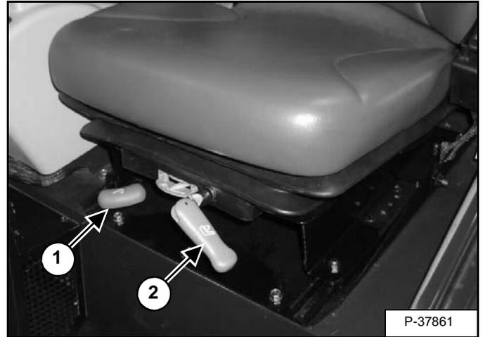
Release the lever (Item 1) [Figure OI-51] to adjust the seat distance from the steering wheel.
