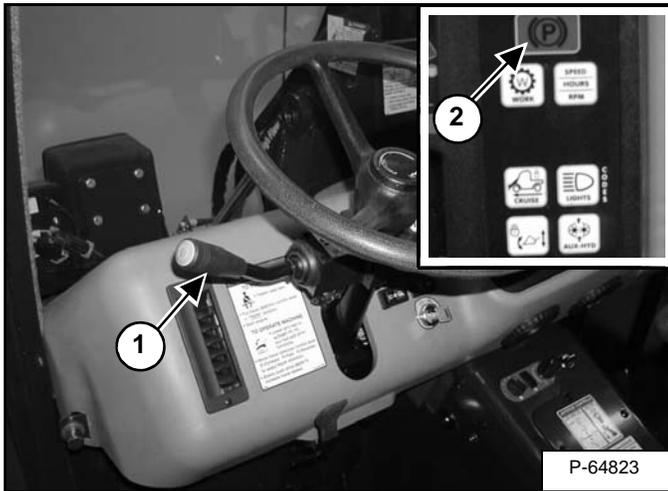
When the Travel Direction Control Lever (Item 1) [Figure PM-11] is in PARK, the Parking Brake is engaged.
