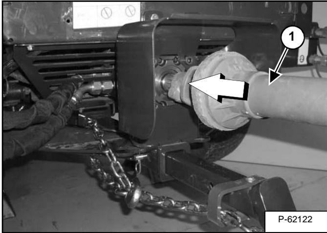
Connect the PTO driveline (Item 1) [Figure OI-34] to the PTO motor shaft. Make sure it is securely connected.
