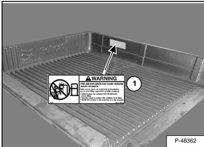
Cargo Box Liner (Option) has a Warning decal (Item 1) [Figure PM-25]. Replace if damaged or missing.
