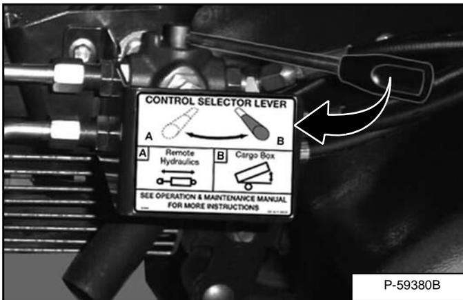
Move the selector lever to position “A” [Figure OI-43] for remote hydraulic operation.
