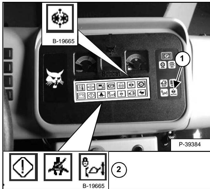
Activate the auxiliary hydraulics (Item 1) [Figure PM-1], raise the arm rest, and verify that the auxiliary hydraulics are deactivated.
