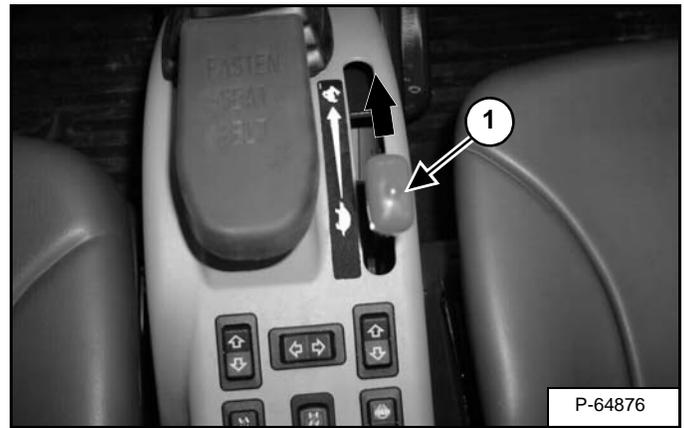
Push the engine speed lever (Item 1) [Figure OI-38] forward to increase engine speed to 2700 RPM (+/- 10 RPM). The engine must be operated at 2700 RPM for 540 RPM PTO operation.
