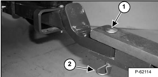
Connect the attachment to the hitch using a hitch pin with a very low or no handle (Item 1) [Figure OI-31]. The hitch pin should be long enough to go through the hitch on the attachment. Install a retaining pin (Item 2) [Figure OI-31].
