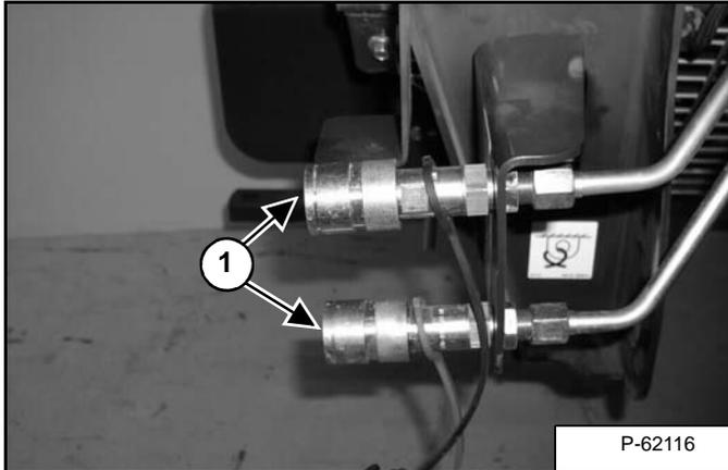
Remove the plugs from the quick couplers. Clean both the male and female couplers (Item 1) [Figure OI-45] before connecting.
