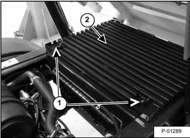
Remove the two debris screen wing nuts (Item 1) and remove the screen (Item 2) [Figure PM-30].
