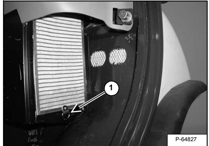
Remove the filter (Item 1) [Figure PM-13] and use a vacuum to clean the evaporator coils.
