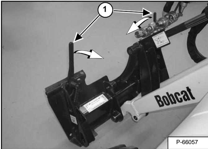
Move the Bob-Tach levers (Item 1) down to engage the wedges [Figure PM-67]. The levers and wedges must move freely.
