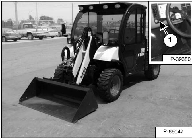
Lower the lift arm, put the attachment flat on the ground [Figure OI-58] and stop the engine.
