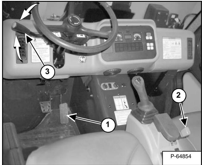
Gradually release pressure on the Drive Pedal (Item 1) [Figure OI-14] until the machine comes to a complete stop.
