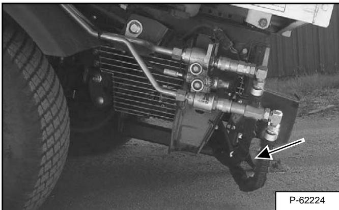
Remove the receiver hitch (if necessary) before loading or unloading to prevent it from hitting the ground [Figure OI-81].
