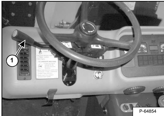
To check the function of the Neutral Start System, place the Travel Direction Control Lever (Item 1) **[Figure PM-5]** in FORWARD and turn the key switch to START position. The engine must not start.
