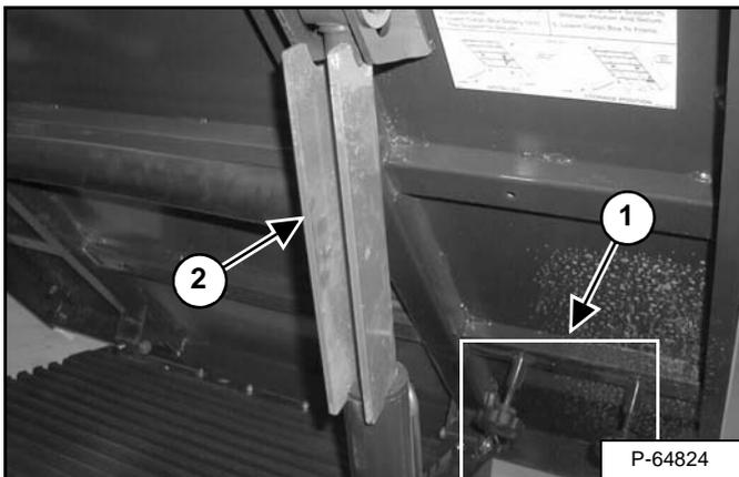
Remove the cargo box support device from the storage position (Item 1) [Figure PM-9].
