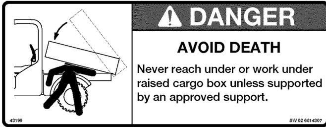
Raise the cargo box and install the approved lift arm support device.
