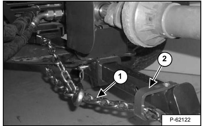
Route the safety chain (Item 1) [Figure OI-32] through the intermediate support (Item 2) [Figure OI-32] and fasten it around the hitch as shown. Allow no more slack in the chain than is necessary for turning.
