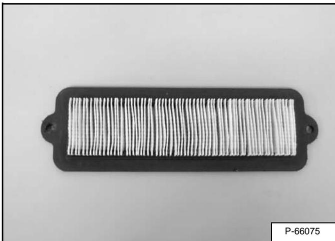
Remove the filter and shake it or use low air pressure to remove dirt [Figure PM-15]. The filter can be cleaned several times in this manner then it must be replaced.
