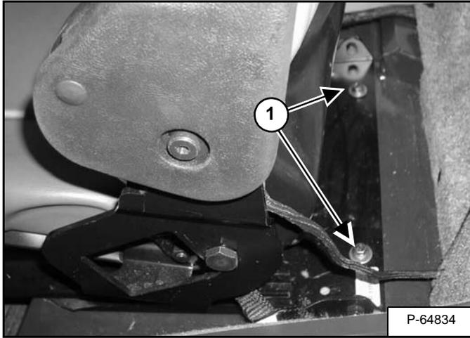
Remove two bolts (Item 1) [Figure PM-20] at the rear edge of the seat pan.
