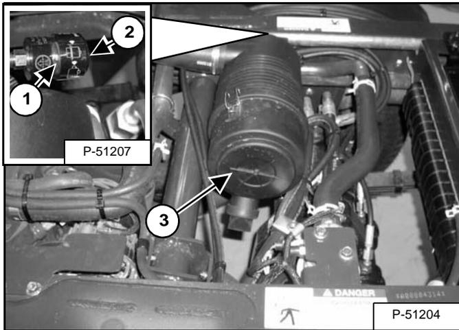
Replace the outer filter element only when the red ring (Item 1) [Figure PM-17] shows in the window of the condition indicator.
