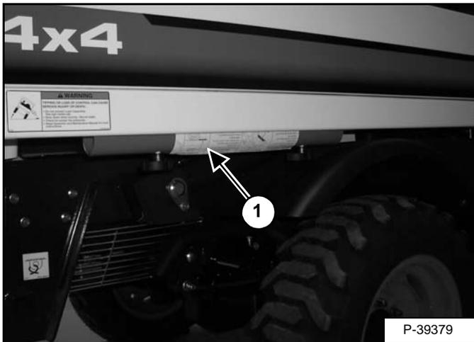
Remove the lift arm support device (Item 1) [Figure PM-6] from the storage position under the right side of the Cargo Box.
